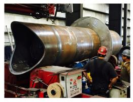
pile cap frames. The pipe was manufactured by TBAILEY and bevel prepared utilizing our custom designed automated burning machine for each of the intricate pipe joints. Some of the sections prepared and joined
